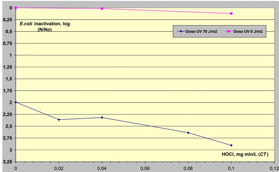
figure 4 : Inactivation of *E. coli* after UV irradiation (70 J/m<sup>2</sup>) followed by HClO (0-0.1 mg/L min).
