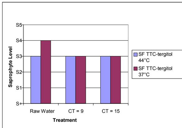
figure 7 : Elimination of SF by Cl<sub>2</sub> with a Ct of 9 and 15 mg.min.L<sup>-1</sup> without UV irradiation.
