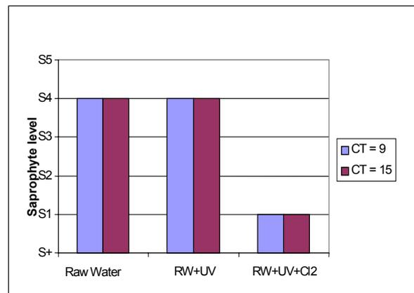
figure 8 : Elimination of the SF with UV only (600Jm<sup>2</sup> m<sup>-2</sup> and UV + Cl<sub>2</sub> (on TTC tergitol, 37°C).
