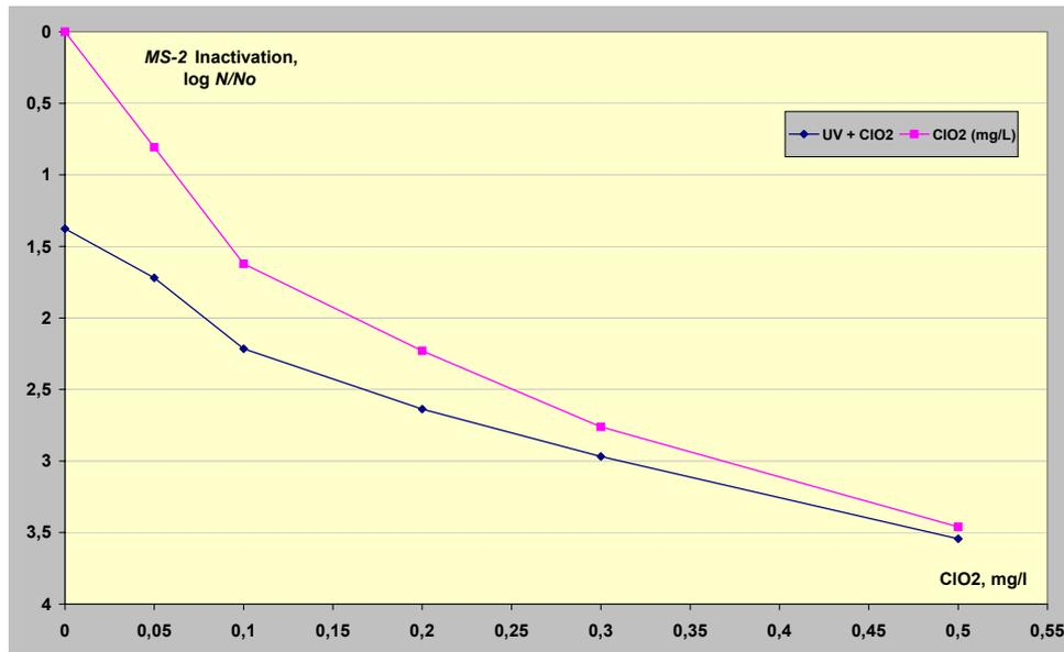
figure 5 : Inactivation of MS-2 after UV irradiation ( $200 \text{ J/m}^2$ ) followed by  $\text{ClO}_2$  (0.05-0.5 mg/L).
