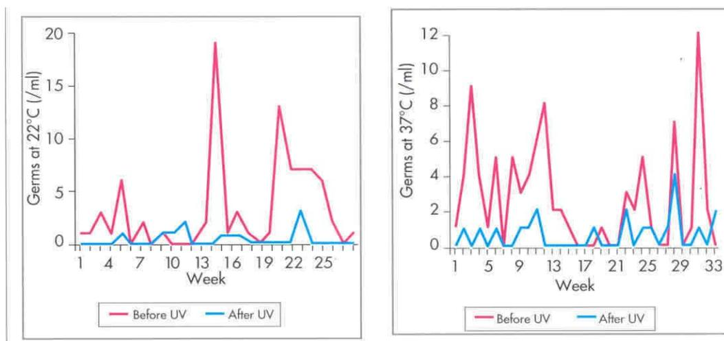
figure 6 : Disinfection results of the system  $\text{ClO}_2$ /UV for HPC (Esparza, 1997).
